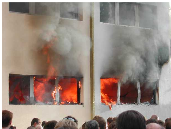
Photo: Façade fire test (after 27 minutes)
