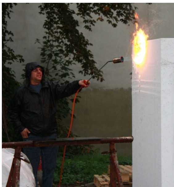
Photo: Block of constructional EPS with flame applied
