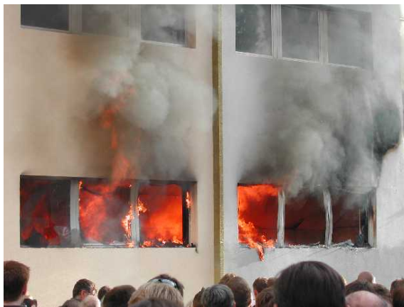
Photo: Façade fire test (after 27 minutes)
